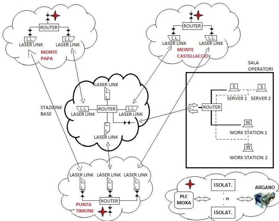
The software installed in the workstation situated in the VLF station control room, controls and monitors the entire antenna system 24/7 by performing actions and receiving signals relating to the working status of the winches and all the other connected hardware systems.
