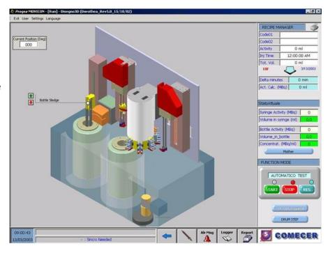
One of the Movicon's screen pages through which the operator can manage the machine.
