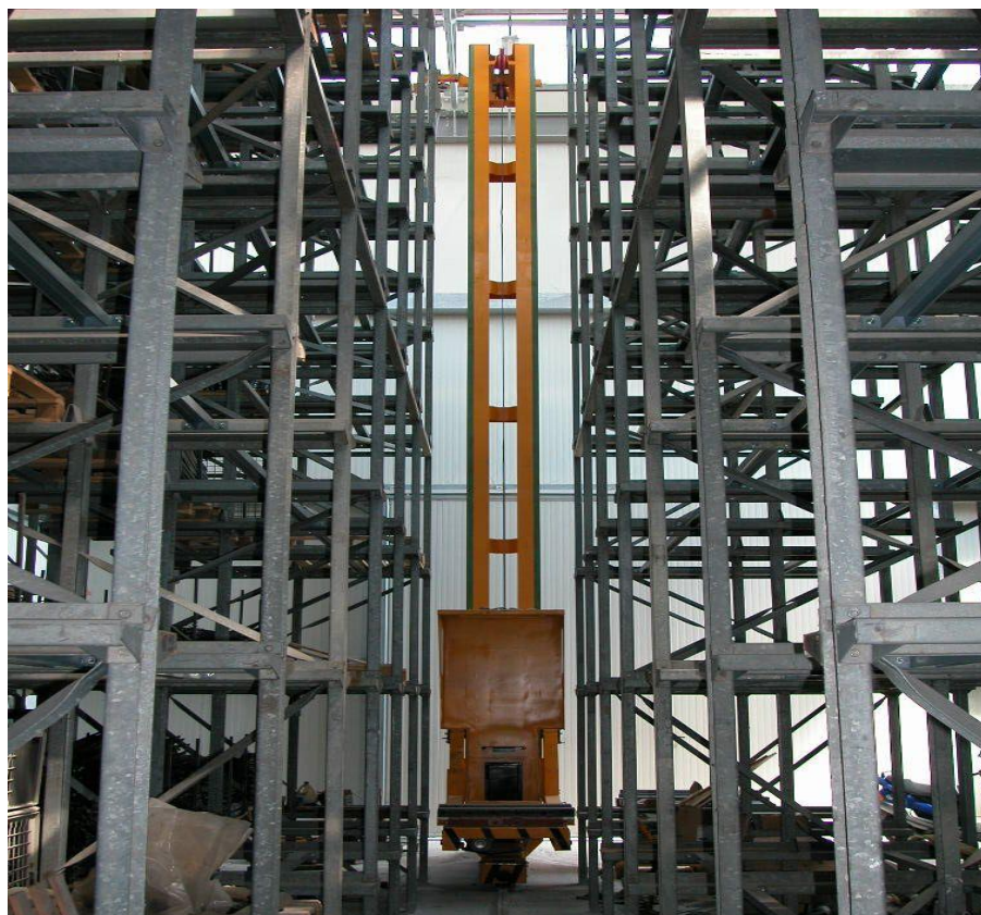
The operator used to manually extract the goods while onboard a shuttle. Now everything has been automated by a system that receives purchase orders from the company management and executes the necessary dispatch procedures all in automatic.
